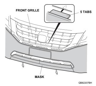
11. Attach the 10 plastic hooks to the top and bottom edges of the front bumper opening.
