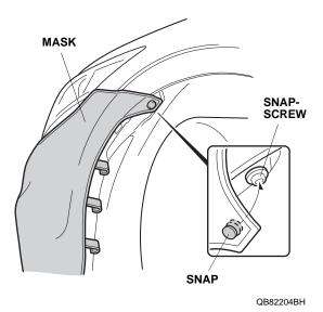
8. Attach six plastic hooks to the fenderwell and the holes of the inner fender. Repeat on the right side.
