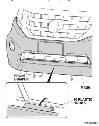
12. Attach two hooks to the bottom of the front bumper.
